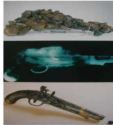
Pistol originally made of cast iron, walnut and brass recovered from the Cygne shipwreck in 1808. The iron, which disappeared, was reconstructed with resin following a mark left on the concretion.
